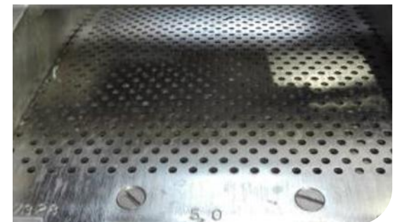
Vibration screen with hole plate (Ø 5 mm)
