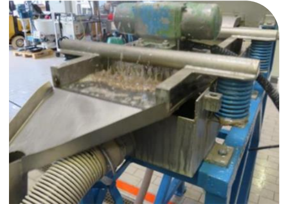
Vibration screen with hole plate (Ø 5 mm)
